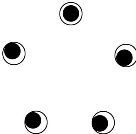
The best procedure is to tighten each lug by hand while wiggling the wheel to ensure that the lugs seat properly in the wheel. Do this a little at a time. If you have to use a lug wrench (or ratchet), just be sure that you very light on the tightening so that if the wheel is off-center, the other lugs can pull it back to center as they are tightened.
